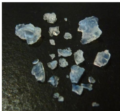
Figure 5. Example of our synthetic common opal synthesized under 0.6 M TEOS condition
