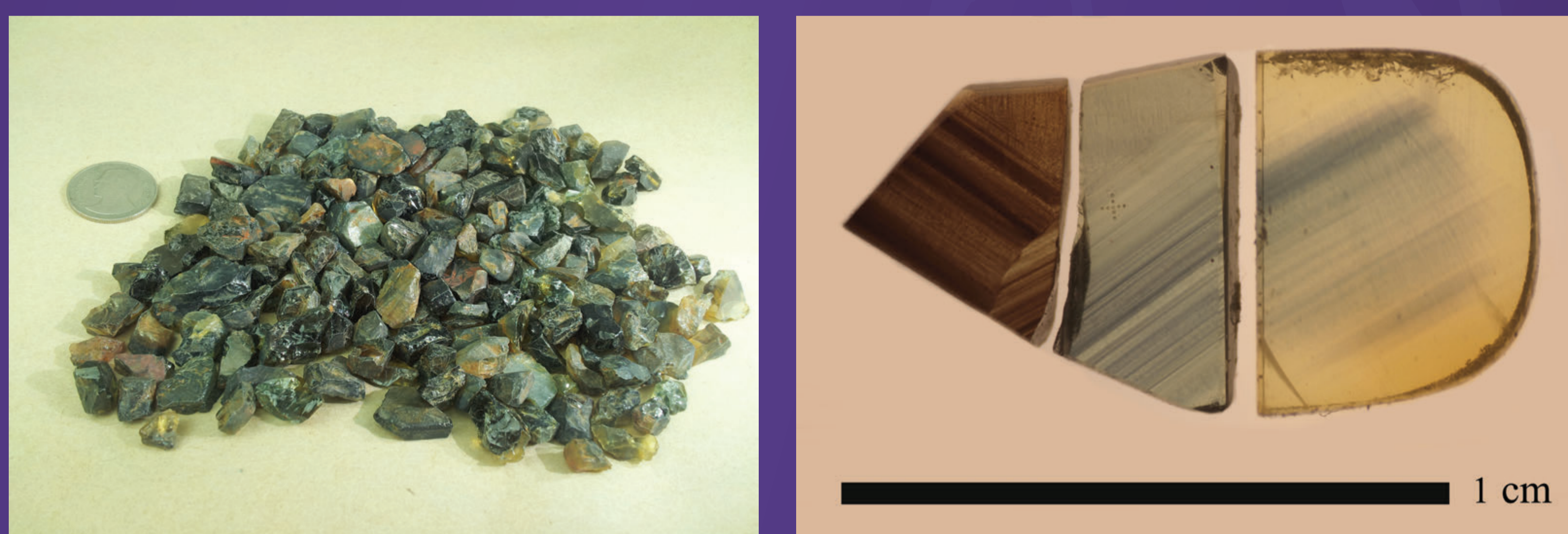
Figure 2. The opaque stones from basaltic deposits in Chanthaburi, Thailand (left) Influence of Be may dissolve the Fe-Ti silks and consequently yield higher transparency and yellow and blue color of the treated stone (right)
